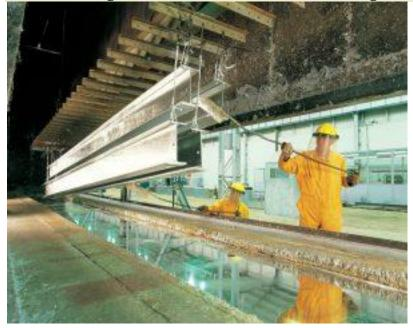
Hot dip galvanizing is the process of coating iron or steel with a layer of zinc by immersing the metal in a bath of molten zinc at a temperature of around 450 °C (842 °F). During the process, a metallurgically bonded coating is formed which protects the steel from harsh environments, whether they be external or internal.
