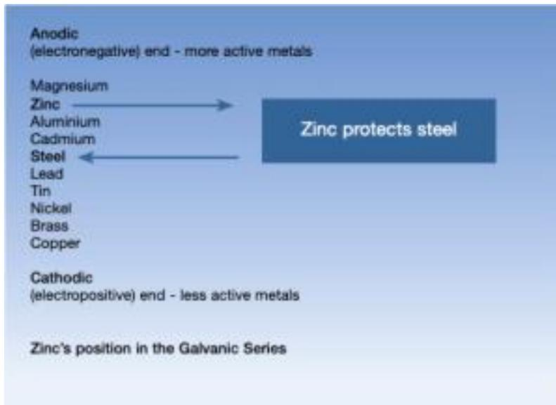
Zinc corrodes in preference to steel and sacrifices itself to protect the steel, hence hot dip galvanizing will provide this **sacrificial protection**.
